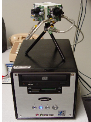
Fig. 1. The CAMEO system consists of a set of FireWire cameras arranged in a panoramic fashion and a small-form-factor PC
