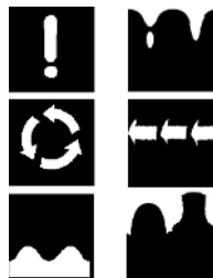
Fig. 1. Some examples of symbols represented in cartesian coordinates (left) and the same symbols represented in polar coordinates (right), using the gravitational center as a pole
