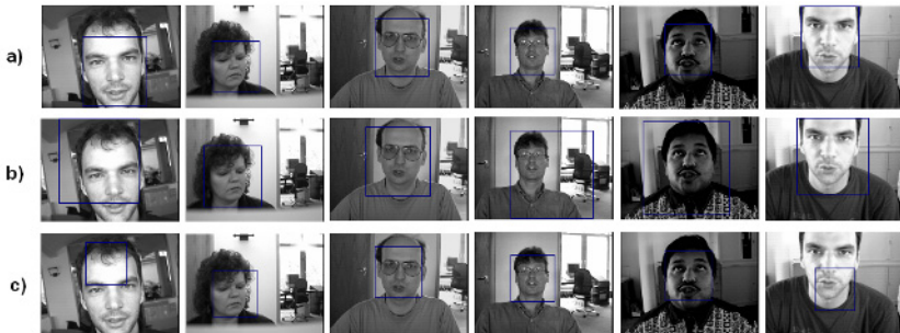
Fig. 8. a) Some examples of correct face detection, including not frontal faces and complex backgrounds, using \sqrt{\frac{s_x+s_y}{2}} as normalization factor. b) Results for the same images using \frac{s_x+s_y}{2} as normalization factor. c) Results for the same images without any normalization factor.
