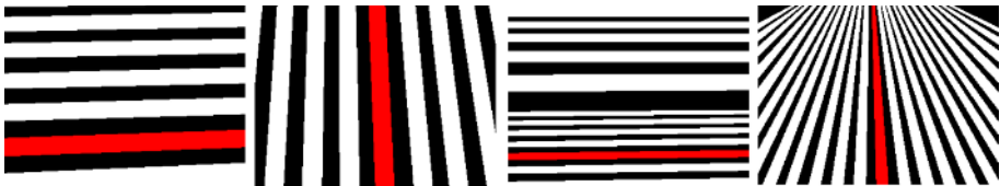
Fig. 6. Horizontal and vertical coordinate calibration images, for 2 different tilt values
